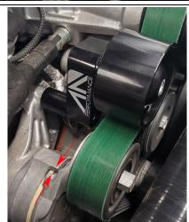
8. The adjustable hole design allows you to swap to a smaller or larger supercharger drive pulley, without changing the drive belt. Most of the time when changing the upper drive pulley it will require you to move which hole the pulley bolts into the bracket.
