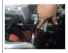
4. Remove the AAD tensioner bracket from the box. Install the M8 and M10 bolts provided into the tensioner.
