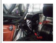
from the box. We recommend installing the pulley in the upper most mounting hole first. This will allow to check the fitment of the belt and the amount of tension on the factory tensioner. Using the 8mm Hex Bit Torque to 35Ftlbs.
