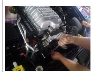
2. Use the 15mm wrench or socket to remove the stud on the front cover assembly.
