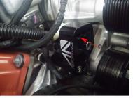
6. Using the 15mm wrench or socket move the factory tensioner back toward the driver side and reinstall the belt.
