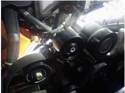
7. You do not want your factory tensioner too tight. This will lead to premature failure for your tensioner and belt. You want the factory tensioner to be in the middle of the travel, the picture included is too tight and will cause issues.
