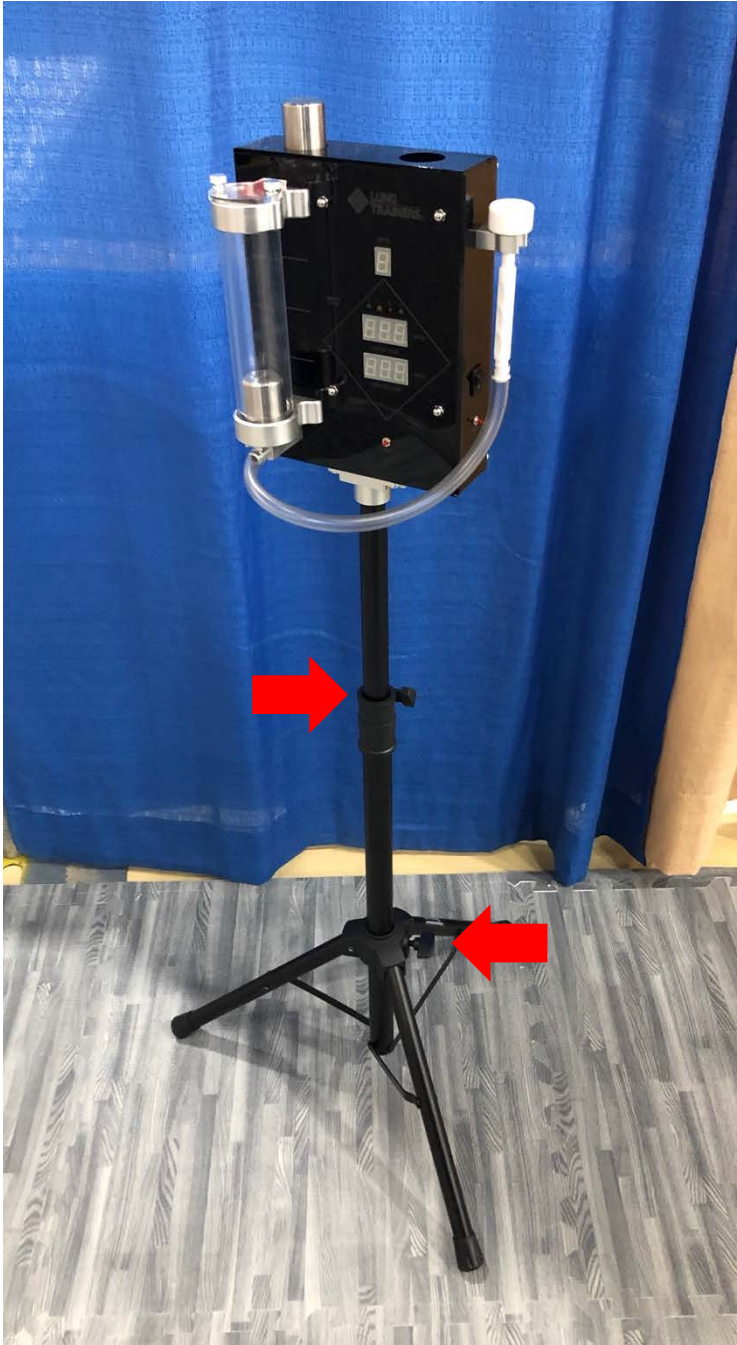
LungTrainer Device Mounted on Floor Stand, Note Position of Hand Screws Identified with Red Arrows
