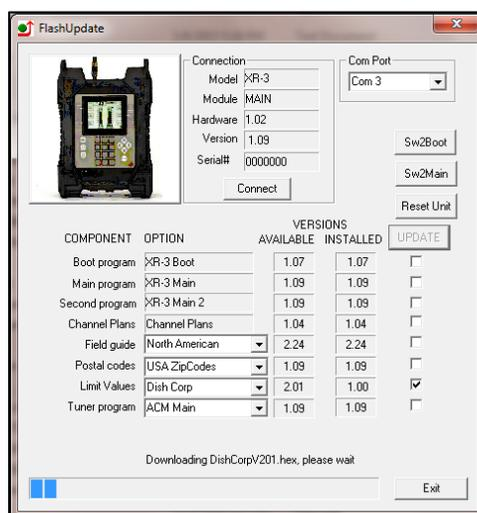
The word "REMOTE" should appear on the LCD screen of the XR-3 to indicate that the instrument is being programmed and controlled remotely. Standby while the instrument is updated. Do NOT press
