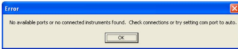
In this case, check to be sure the instrument is on and the USB data transfer cable is fully seated. Click "Connect" to retry the connection. With the USB connection, the computer should automatically establish connection with the meter. If you don't know the com port number, you can choose Auto or try all available ports or you can check your COM port assignments in the Device Manager section of the Windows Control Panel.
