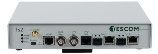
Mobile operators are deploying small cells to build out their LTE and 5G networks. This is occurring in a variety of locations such as in urban canyons and indoors, where GNSS signals are weak or intermittent. TesCom's Ts2, a multi-sync gateway addresses the challenges of providing reliable and precise synchronization everywhere through IEEE 1588-2008 (PTP) and leveraging multiple sync references.
