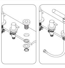
Disassemble the cold water handle (1) (identified by a blue dot). Leave the bottom retainer ring as well as the rubber and metal washers in place. From under the bathtub insert the cold water valve (indentified by a C) in the hole located on the right of the spout hole.
