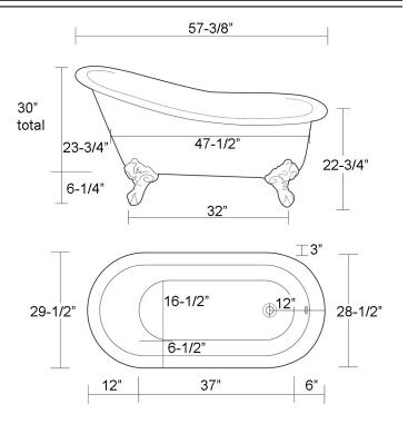
Dimensions of fixture are nominal and may vary within the range of tolerances established by ANSI Standard A112.19.1M. Dimensions and specifications subject to change without notice.
