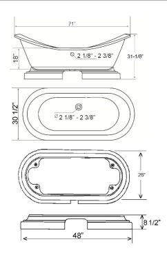
Dimensions of fixture are nominal and may vary within the range of tolerances established by ANSI Standard A112.19.2. Dimensions and specifications subject to change without notice.
