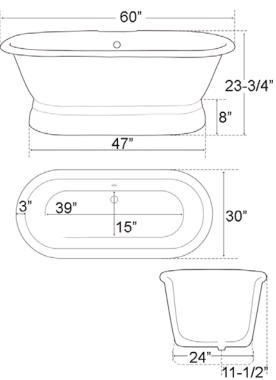
Dimensions of fixture are nominal and may vary within the range of tolerances established by ANSI Standard A112.19.2. Dimensions and specifications subject to change without notice.
