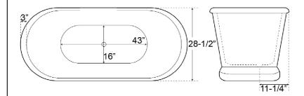
Dimensions of fixture are nominal and may vary within the range of tolerances established by ANSI Standard A112.19.2. Dimensions and specifications subject to change without notice.
