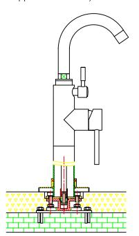
4.After connecting the water pipe with the connection seat(4), make the water trial while turn on the switch. Invaginate the connection seat(4) to the plastic guard(4) after make sure to be without leakage. Then, as shown on the above Fig, spread the decorative floor.
