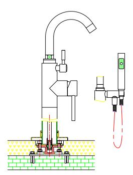
7.Connect the Flexible hose(8) and handle shower (9)with Main body Assembly(1), and place the Shower handle(9) on the Shower Hook.
