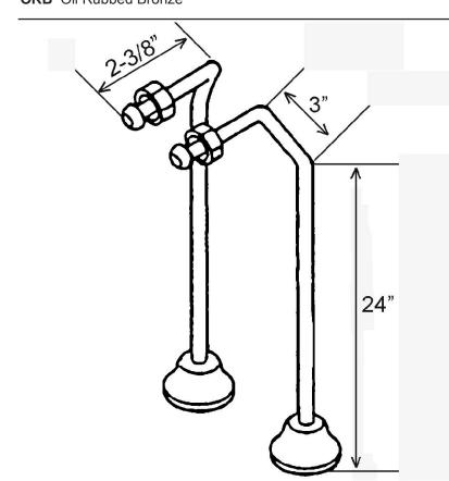
Use on concrete floors requires special installation. We recommend using a plumbing proffessional.
