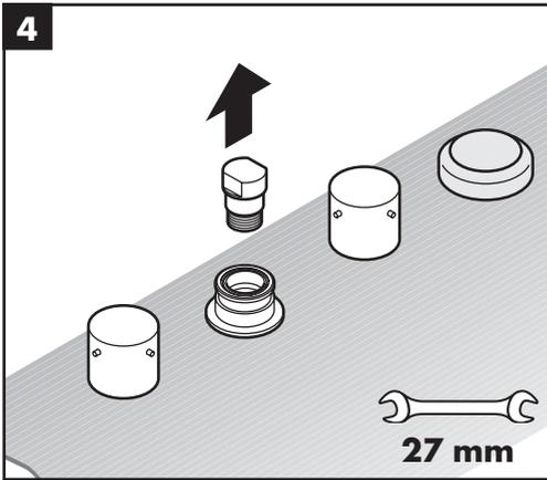
Remove the plug from the diverter housing.
