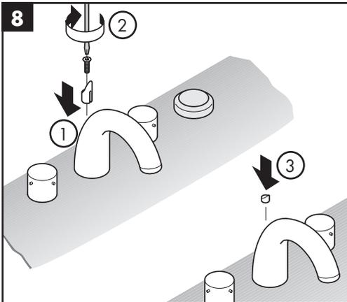
Install the diverter knob, screw, and screw cover.
