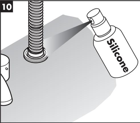
Lubricate the Secuflex hose using silicone spray.
