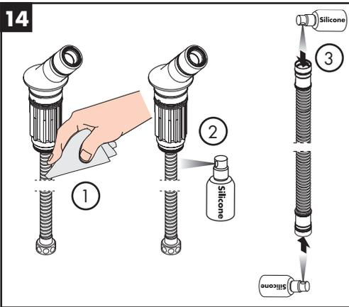
Lubricate the handshower hose using silicone spray.
