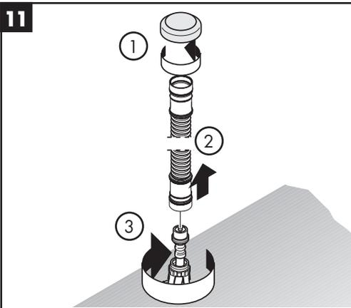
(1) Remove the plaster shield from the Secuflex hose.
