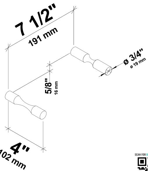
Vino Pins Flex Magnum spacing adds 1" (26mm) to the installation width.
