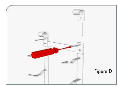
**Option 1** - If stacking multiple units, do not install the decorative scrolls in the lower units. Instead, slide the bottoms of the upper racks into the gap behind the top of the lower rack. For the upper units, the Lower Cross Rail is not used and may be discarded.
