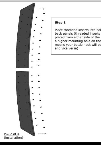
Place threaded inserts into holes in back panels (threaded inserts can be placed from either side of the panel, a higher mounting hole on the right means your bottle neck will point right,
