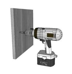
Faster Installation Method: Fit the anchor bolt into an electric drill and screw into your pilot hole. Be careful not to screw too deep. Leave sufficient bolt length sticking out of the wall for mounting the peg.
