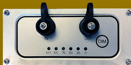
Onboard Dimmer & External Dimming connections
