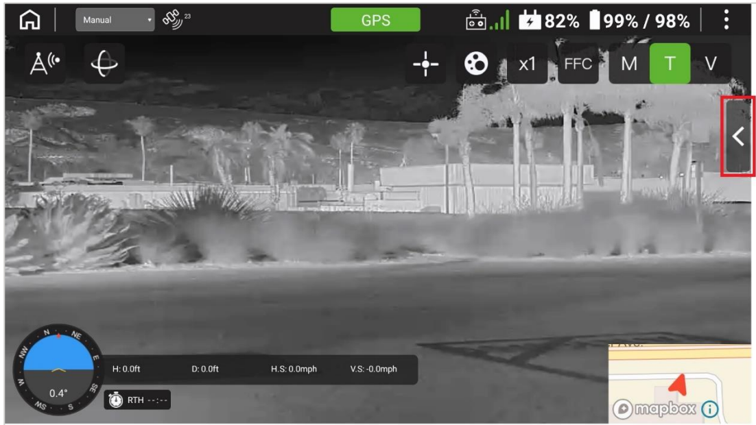
FIGURE 7.U BUTTON TO EXPOSE HIDDEN SHUTTER CONTROLS
