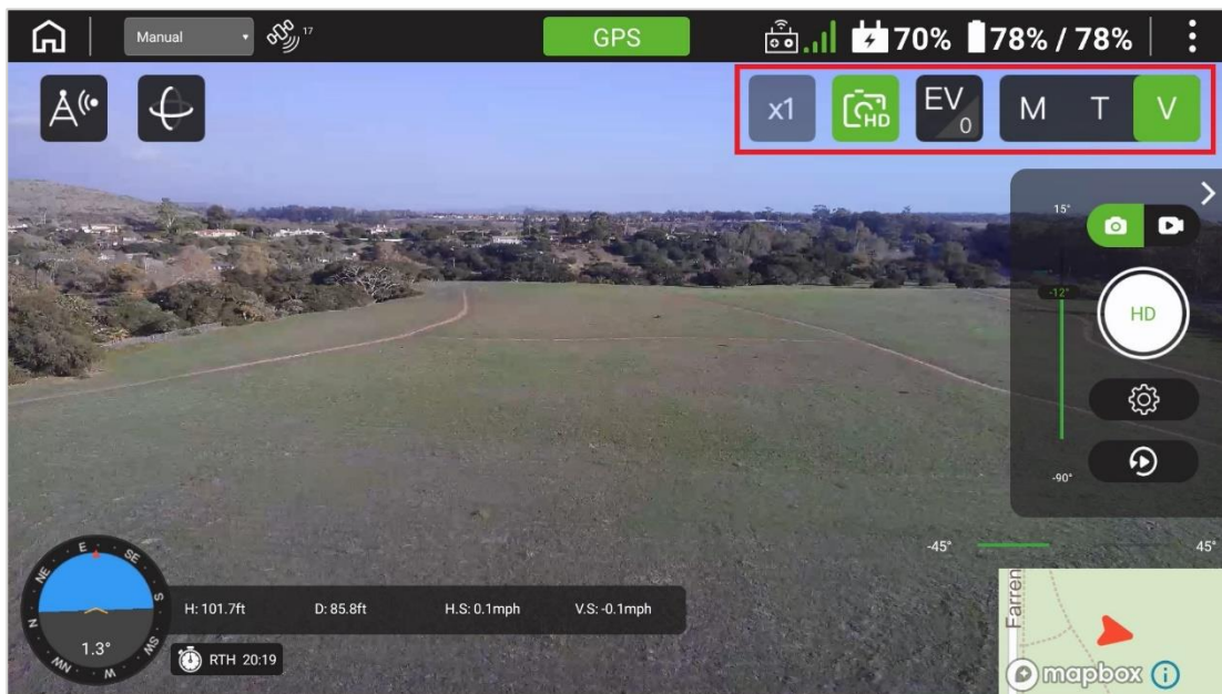
FIGURE 7.O VISIBLE CAMERA QUICK-ACCESS FEATURES
