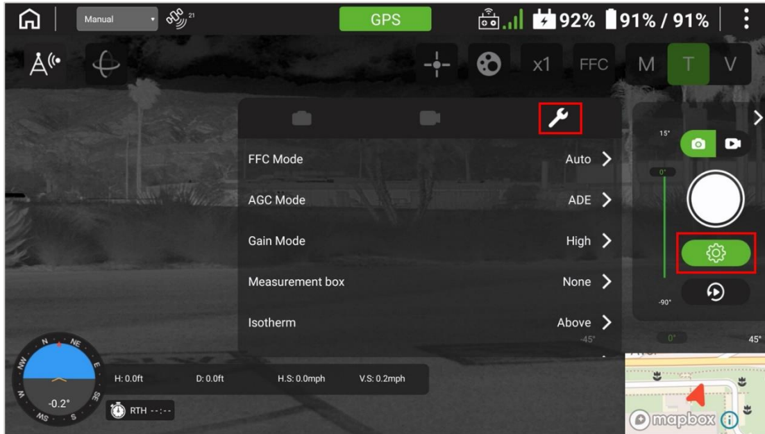
FIGURE 7.Y RADIOMETRIC ADJUSTMENTS FOR THERMAL CAMERA
