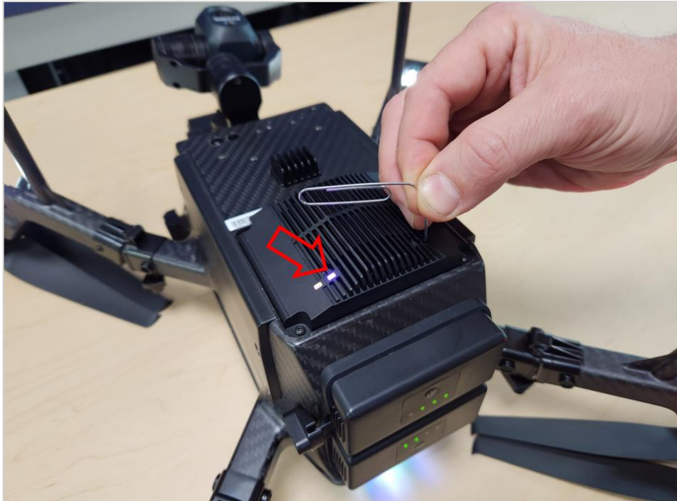
FIGURE 7.J PRESSING THE PAIR BUTTON (PAIRING LIGHT FLASHING)
