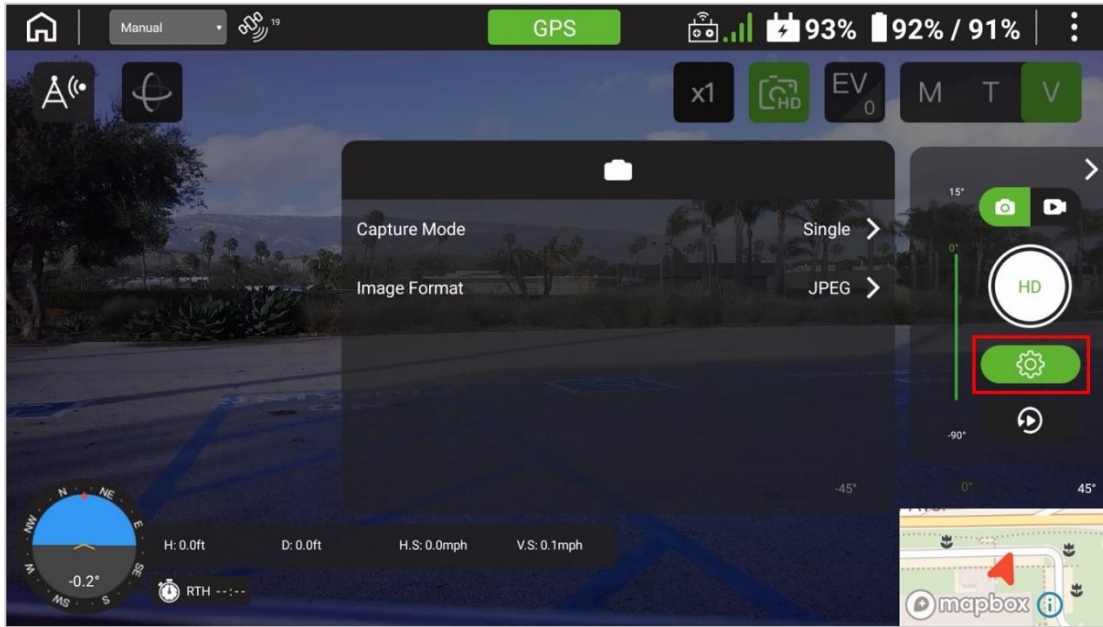
FIGURE 7.V CAPTURE MODE AND IMAGE FORMAT SETTINGS FOR VISIBLE CAMERA
