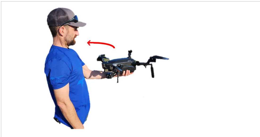
FIGURE 8.B COMPASS CALIBRATION STEP 2: HORIZONTAL ROTATION, LEVEL
