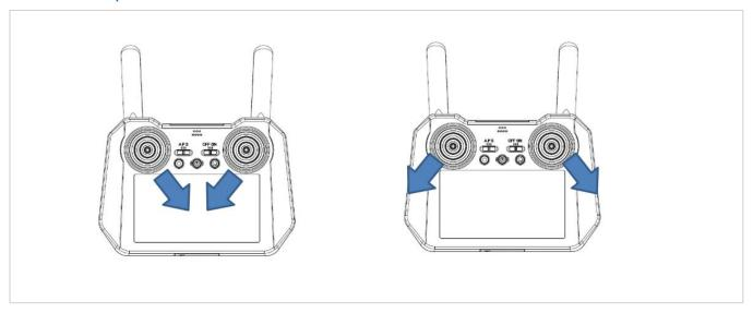
Pull both joysticks backward and in to start the motors. Push the left joystick forward to take off. Pull both joysticks back and apart to stop the motors.
