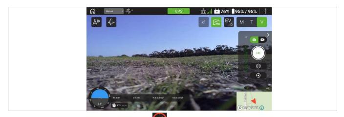
If the main display shows the Calibrate Compass ( icon in the top bar, the compass must be calibrated. See the *User Manual* for instructions.
