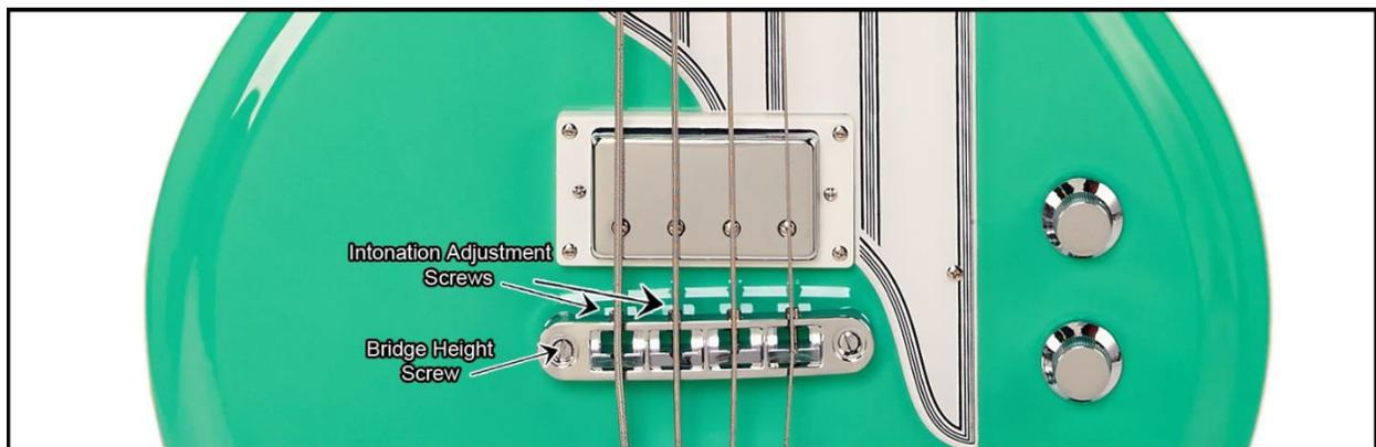
**PICKUP HEIGHT:** This refers to the distance between the bottom of your strings and the top of the pole pieces in the pickups. These should be set properly so that your strings have equal output, and the guitar's tone is represented as it should. That said, the following measurements are guidelines only, and
