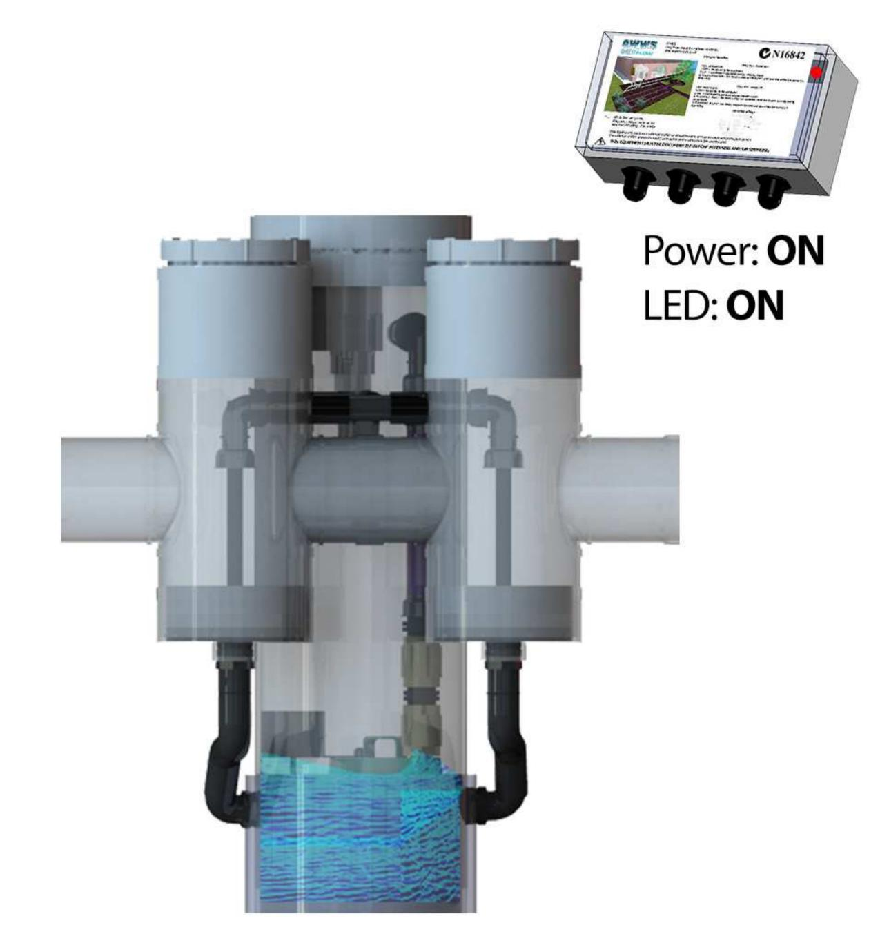
Water level in the main pit is below the float switch level
