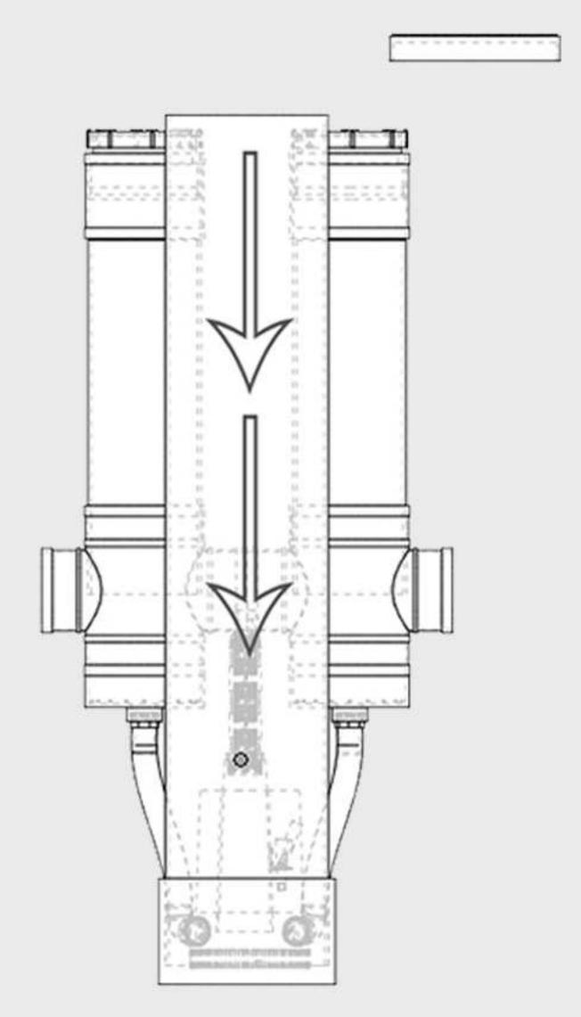
Secure the pump on the bottom of the pit
