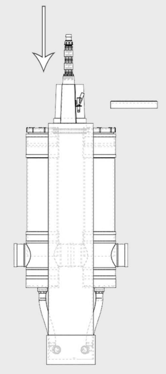
Install the pump all the way into the 250mm PVC pit
