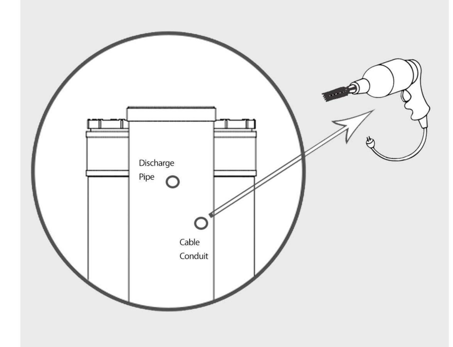
8. Run cable through electrical conduit to wall mounted powerpoint
