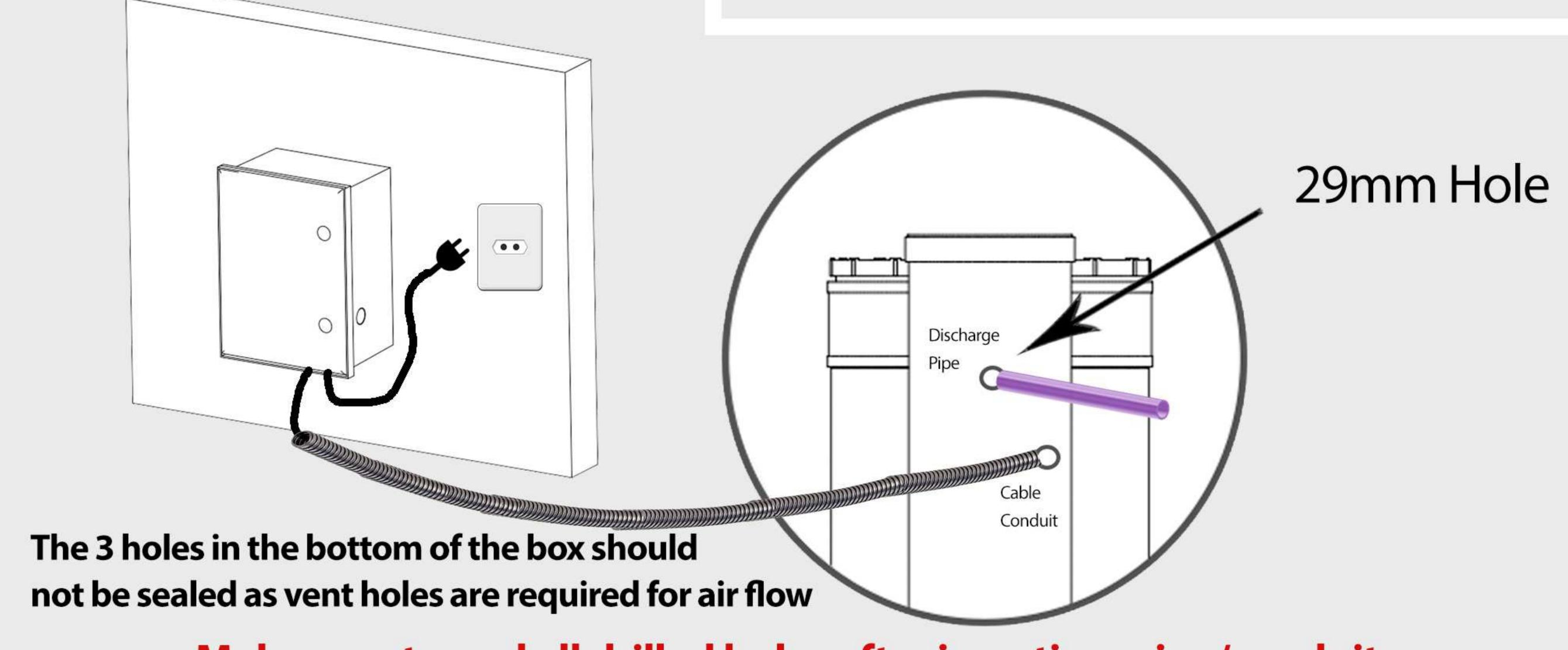
Make sure to seal all drilled holes after inserting pipe/conduit
