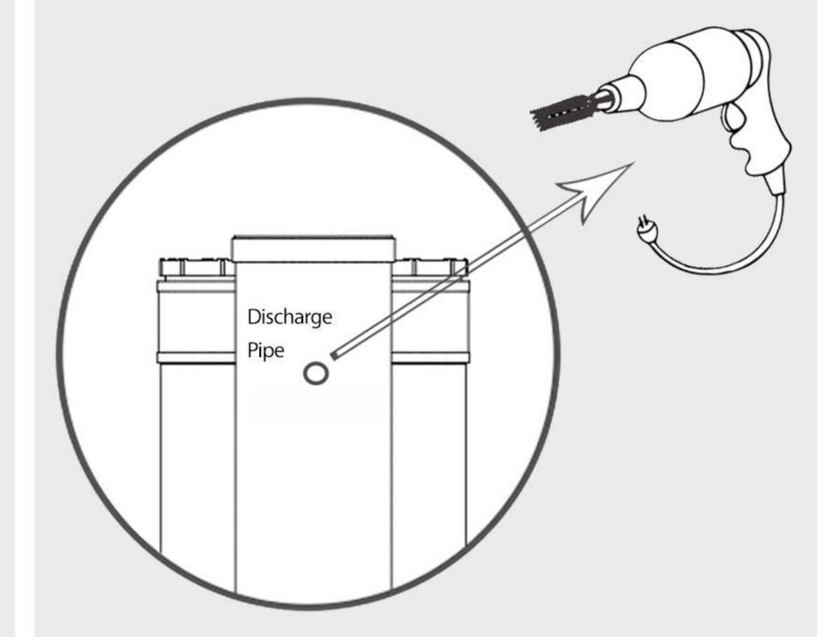
With 25mm low density poly pipe a 29mm hole is required
