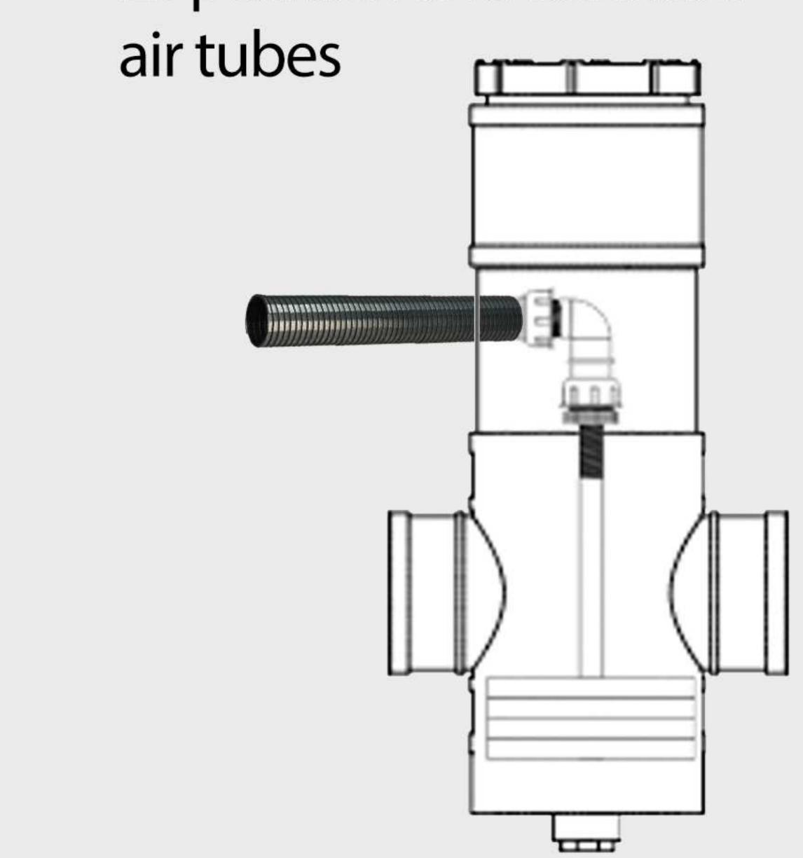
14. Run 25mm low density poly pipe from air blowers to filters
