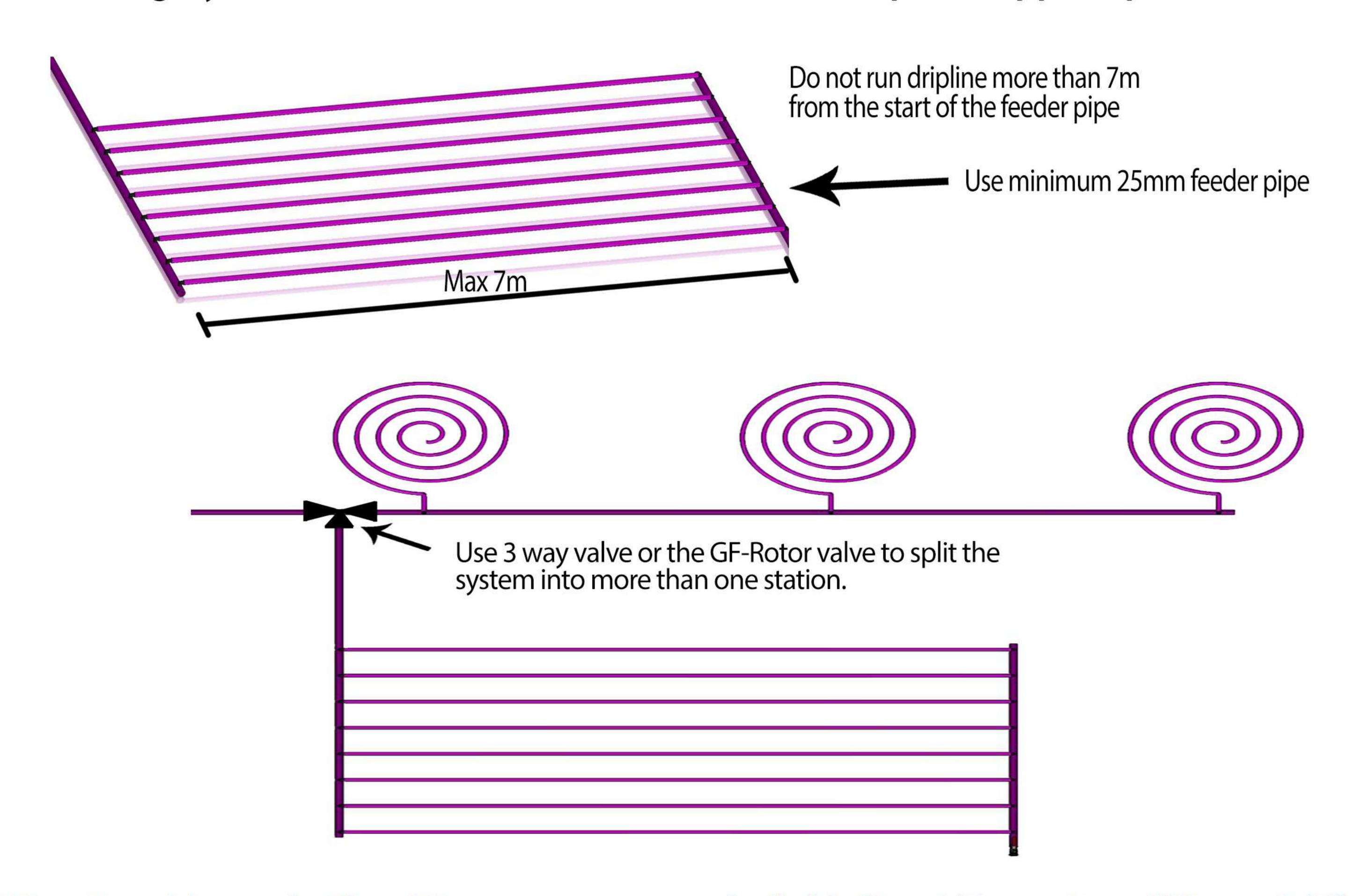
Warning: Use only GreyFLow recommended dripline. Warranty will be void if non-recommended dripline is used. Do not use more than 100m of dripline per station.
