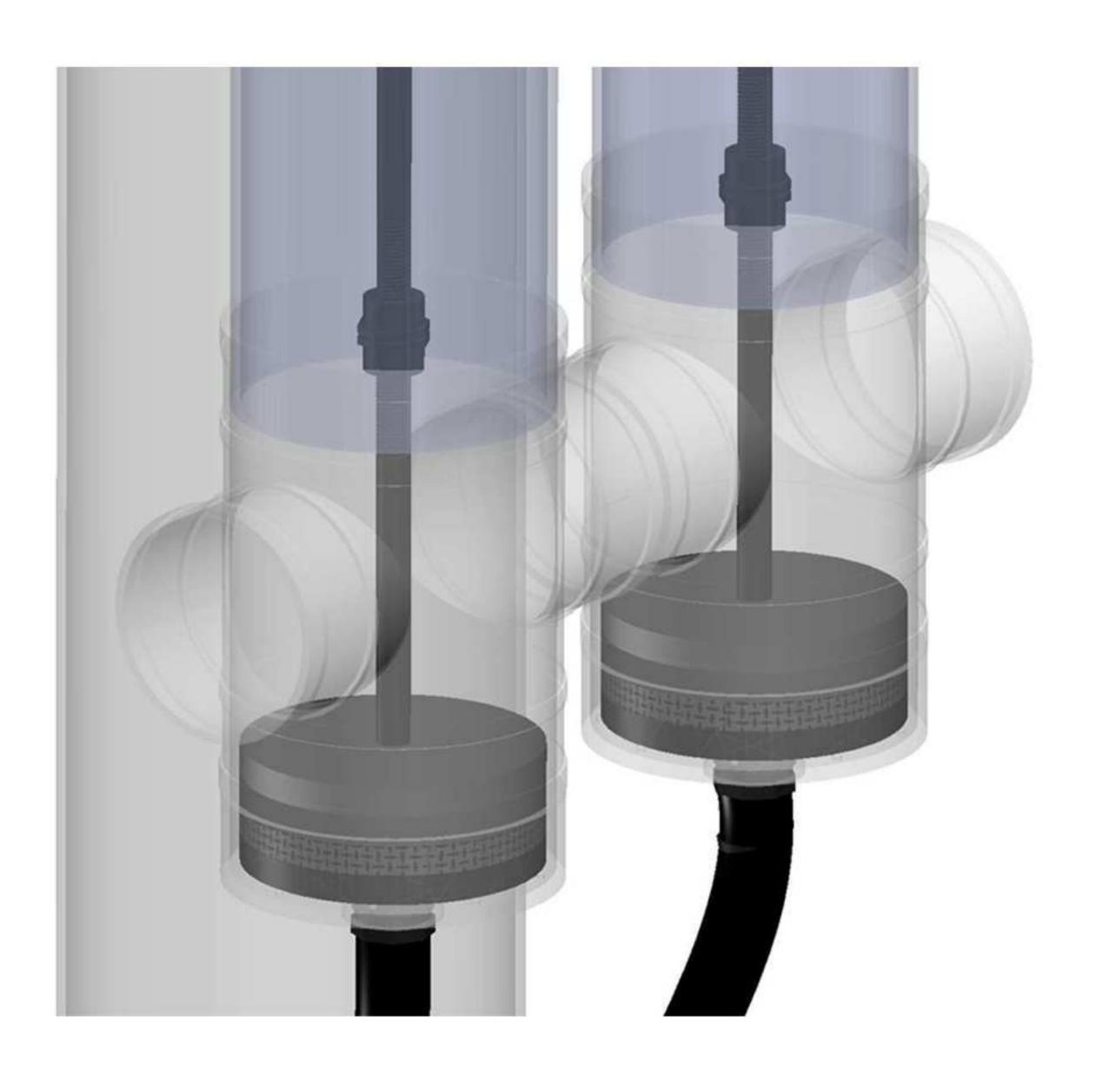
Make sure to insert filters all the way down to the bottom of the interceptor (the filter 1/2" risers should be standing vertically)
