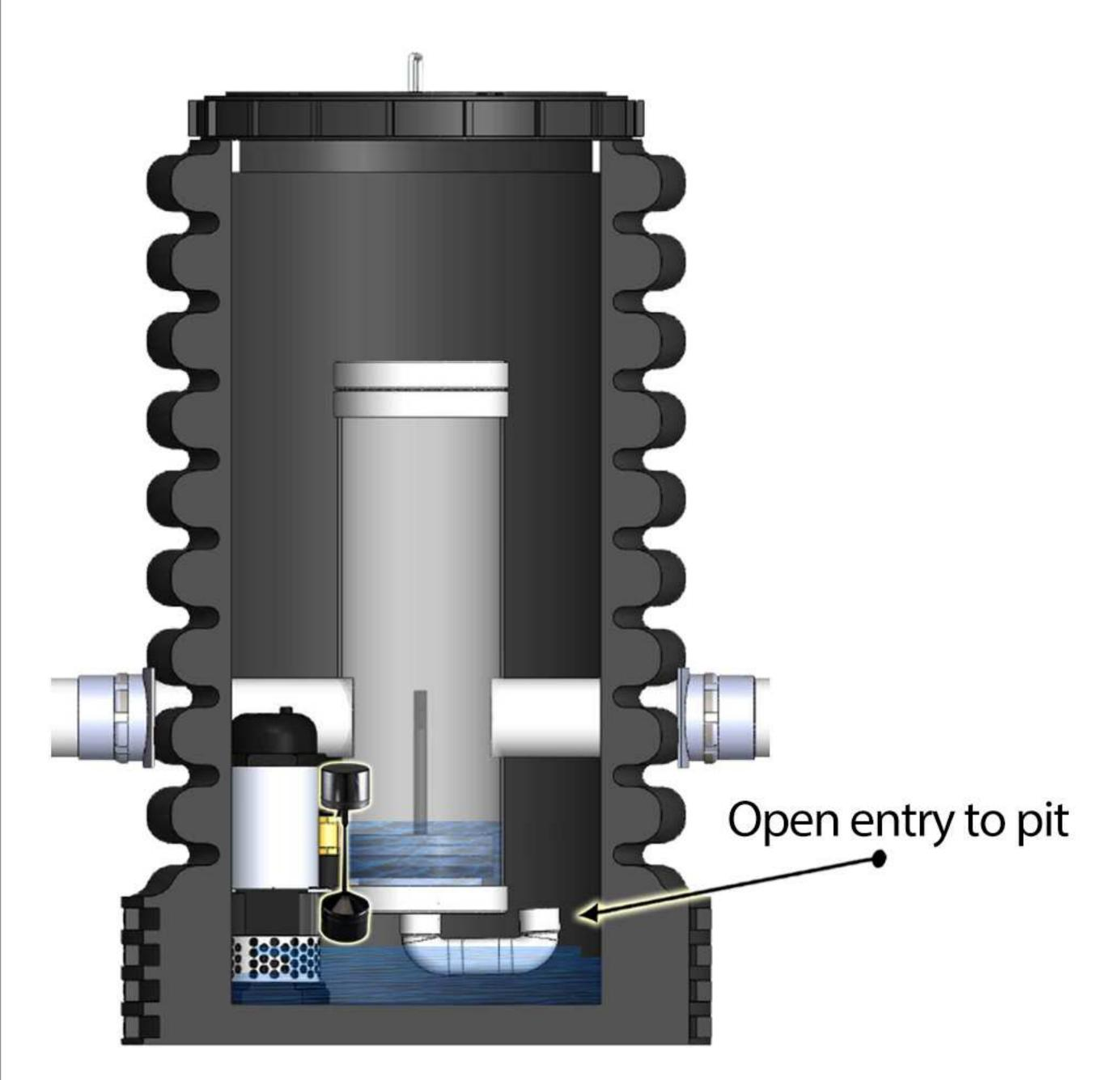
Water level in the main pit is below the float switch trigger level
