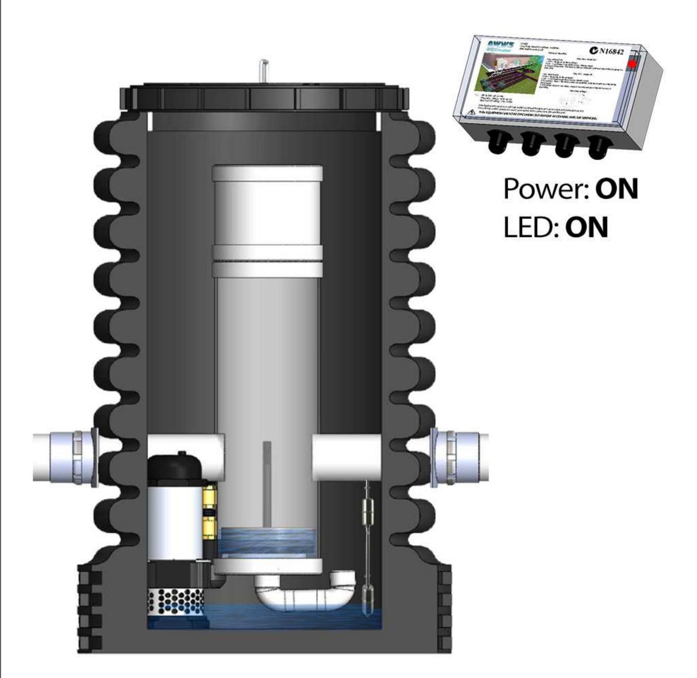
Water level in the main pit is below the FS1 float switch level
