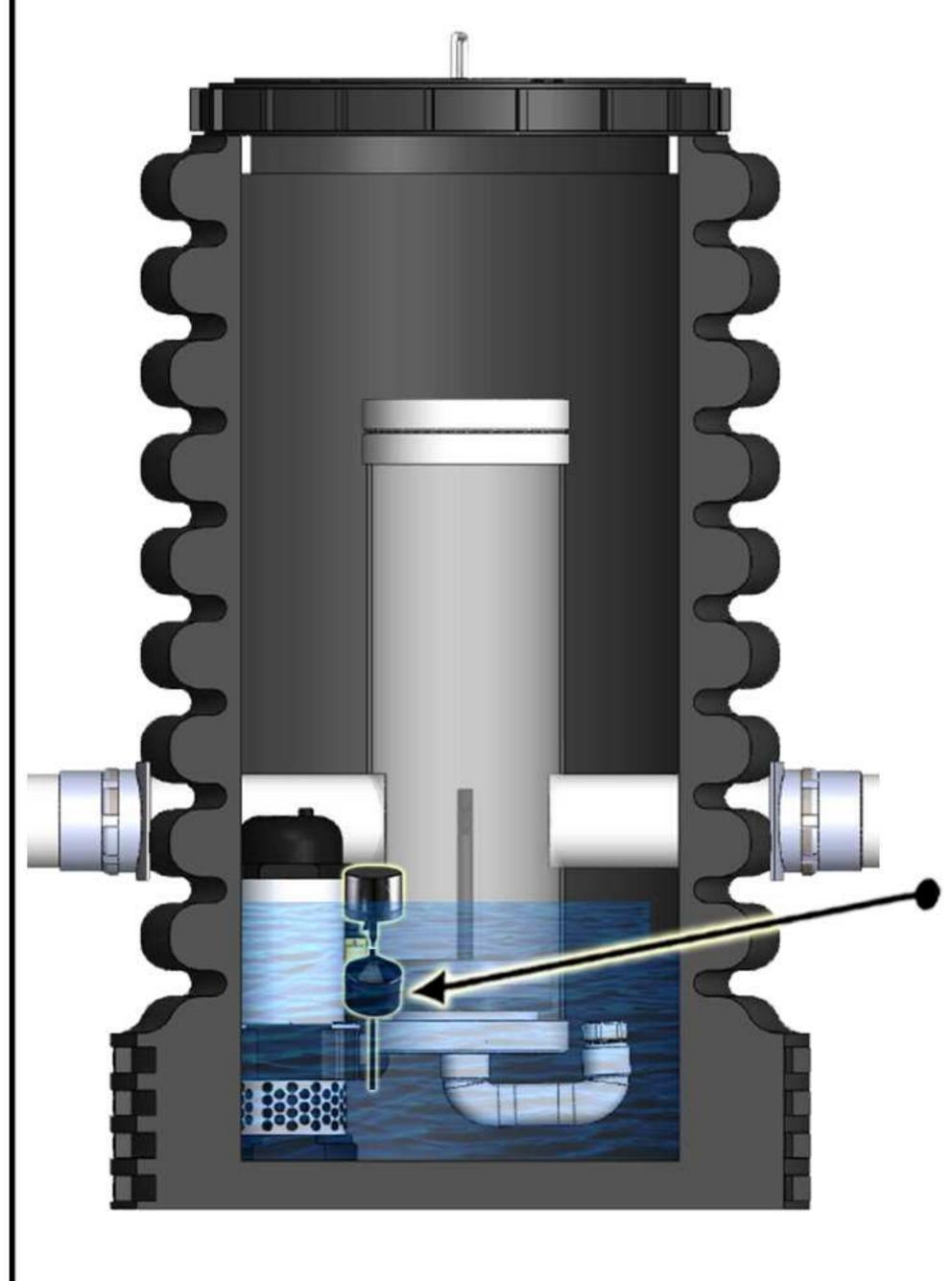
The float switch has reached its trigger point and the pump is discharging the greywater into the irrigation system
