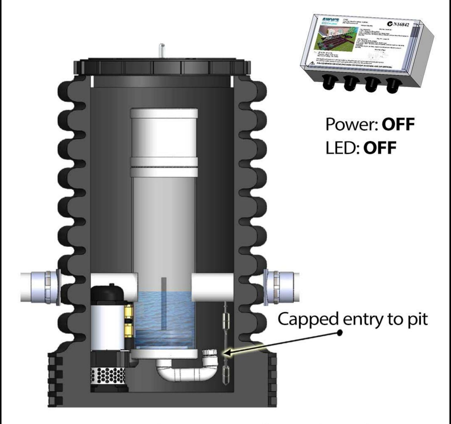
Water enters the system from the inlet pipe, and exits via the overflow pipe
