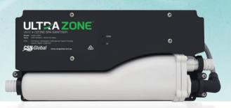
**Ozone is** a naturally occurring oxidiser created in the UltraZone® unit using a corona discharge. This ozone is then injected and mixed into the patent pending UV chamber. The UV then reacts with the ozone to create a powerful oxidiser to burn off unwanted organic matter – the result, crystal clear, clean water.
