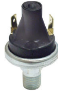
KEY OEM REF DESCRIPTION MAK1MR2414A SWITCH, Low Pressure 1/4in P.T. Normally Closed (0 psig) Opens at 70 psig(CH Model) Fully adjustable to 5 psig No Lock-Tite Clockwise Decrease
