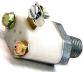
KEY OEM REF DESCRIPTION 745-279416 SWITCH, Low Pressure 1/4in P.T. Normally Closed (0 psig) Opens at 60 psig
