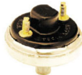
KEY OEM REF DESCRIPTION MAK1MR2225 SWITCH, Low Pressure 1/8in P.T. Normally Closed (0 psig) Opens at 55 psig
