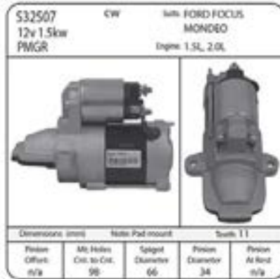
S32507 STARTER SUIT FORD FOCUS/ MONDEO 12V CW 11TH 1.5KW Manufacturer: Ford
