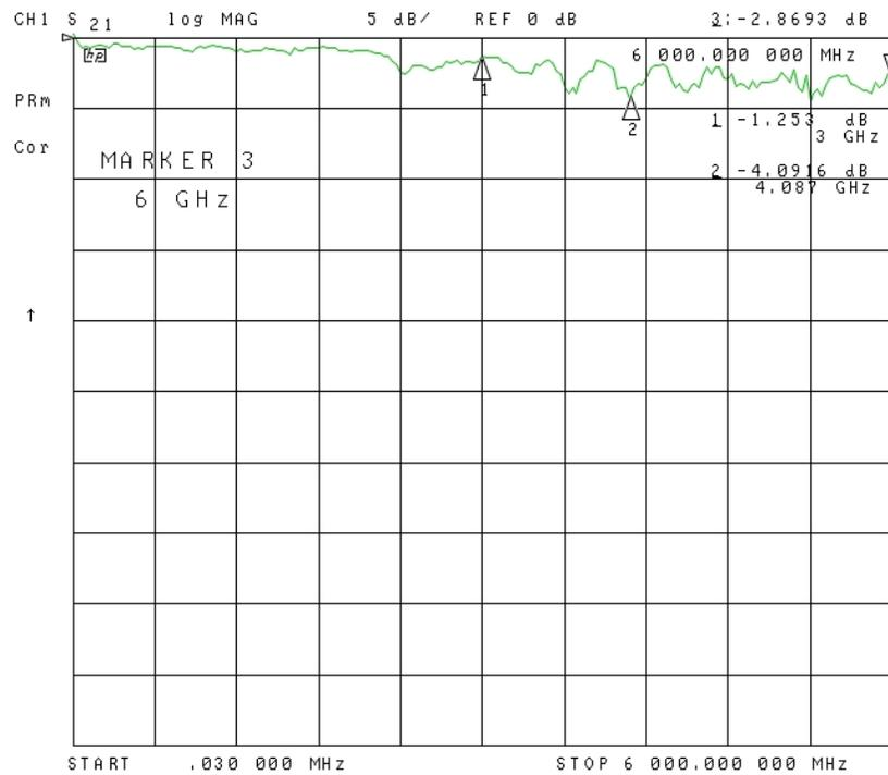
Picture 7 – TBTC0, transmission loss
