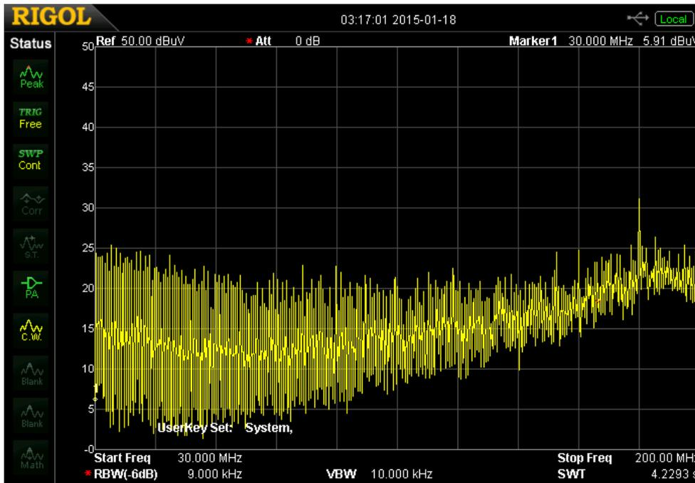
Picture 4 – TBTC1, radiated emissions of a LED lamp prototype after modification. The spurious level in the measured frequency range could be reduced by 10dB $\mu$ V. The spurious crossing 30dB $\mu$ V was identified as picked up from outside.
