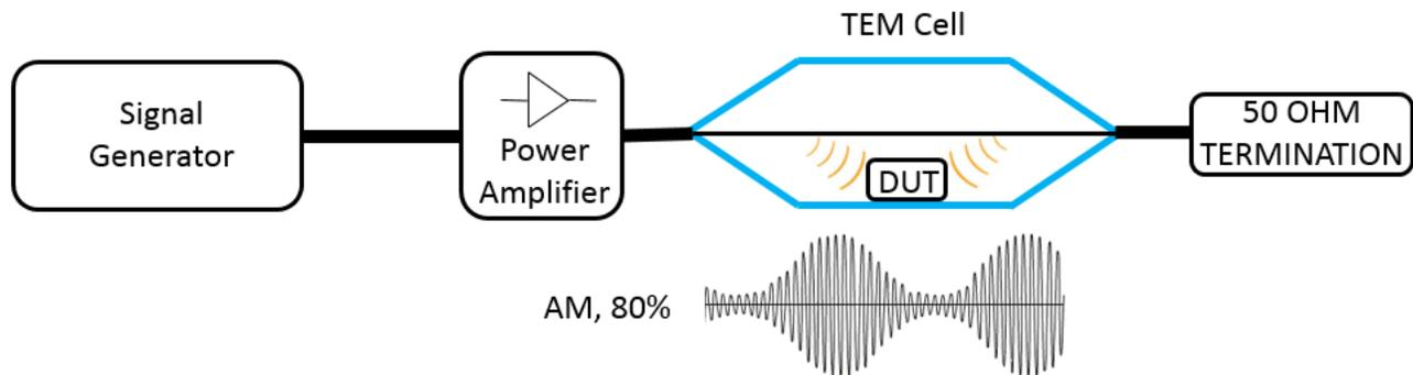
Picture 5 – RF immunity measurement set up
