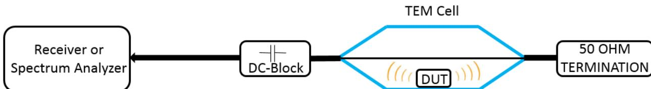
Picture 2 – radiated emission measurement set up
