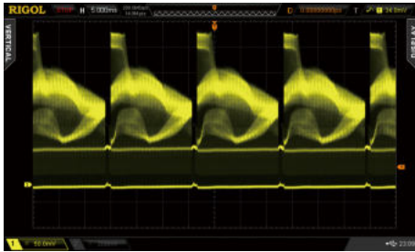
256-level intensity grading waveform display
