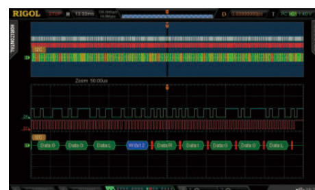
Serial bus triggers and decodes
