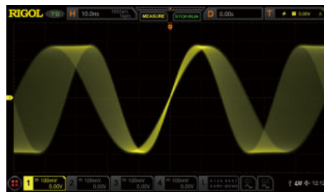
Changes of each frame of waveforms of the sweep signal can be clearly observed in the highly refresh mode.
