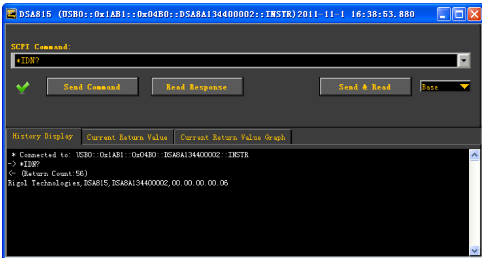
Figure 3-3 Write and Read Commands via USB
