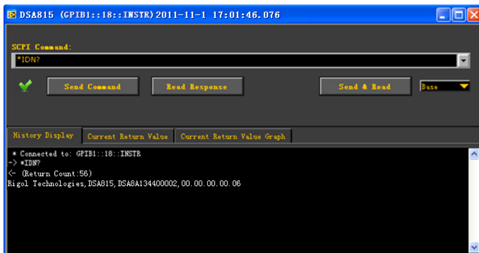
Figure 3-10 Write and Read Commands via GPIB
