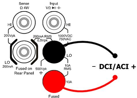
**Note:** in order to protect the multimeter, please execute DC/AC current measurement following the requirements below.
