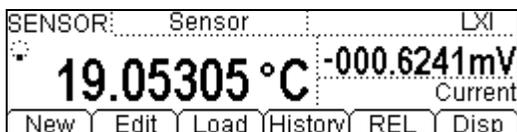
The following part introduces how to create a sensor configuration file in details. For DCV, DCI, 2WR, 4WR or FREQ sensor, you can define a fitting curve. Since the temperature sensor (TC, RTD, THERM) converts the electrical signal (such as voltage or resistance) to temperature using the software conversion program inside the instrument, you can directly choose a desired temperature sensor.
