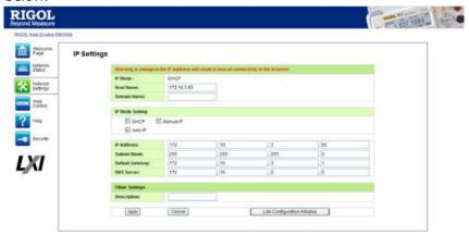
Set the IP via this interface, press "Apply" to enable the modification and press "Cancel" to disable this setting. To restore to factory setting, press "LAN Configuration Initialize".
