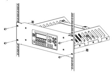
7. Post-installation note: the rack holds a height of 3U. Holes pointed out by the arrows are the installation holes and should be aligned with when installing.
