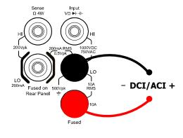
**Note:** in order to protect the multimeter, please execute DC/AC current measurement following the requirements below.
