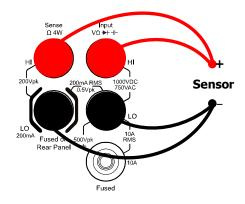
**Note\*:** before setting the parameters for DCI sensor when using it, please connect it according to the figure above and press  $\xrightarrow{\square}$   $\rightarrow$  mA.
