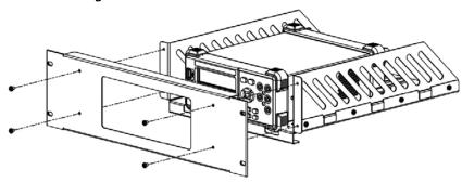
Load into machine cabinet: mount the rack with instrument onto a standard 19-inch machine cabinet using four M6 screws and four M6 square nuts, respectively.
