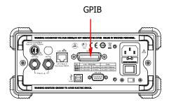
Press  $\bigcirc$  I/O  $\rightarrow$  GPIB to enter the GPIB address configuration interface.
