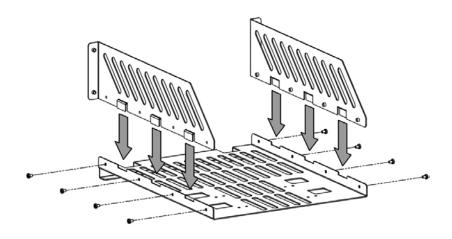
3. Place the instrument: aim the parallels at the corresponding openings and then put the multimeter onto the support board.
