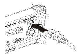
Figure 1-7 Connect the Power Cord
