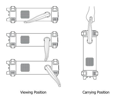
Figure 1-2 Place the Multimeter
