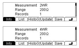
Press Info and use the up and down direction keys to view the measurement item, measurement range, number of values, maximum,
