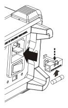
Figure 1-8 Replace the Power Fuse
