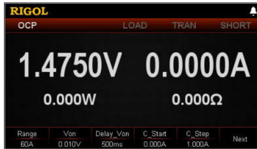
Figure 2-30 Main Interface of OCP Test Function
