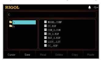
The load allows you to save different types of files to the internal and external memories. You can recall and read them when necessary.
