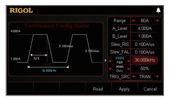
Transient test function enables the load to periodically switch between two set levels (Level A and Level B). It can be used to test the transient characteristics of the DUT. The highest frequency can be set to 30 kHz. Besides, in the guide interface, you can configure parameters in the parameter configuration list and view the configuration diagram at the left of the configuration list in the real-time manner.
