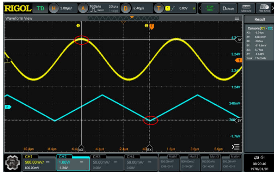
Figure 10.13 Track Measurement (after Horizontal Expansion)
