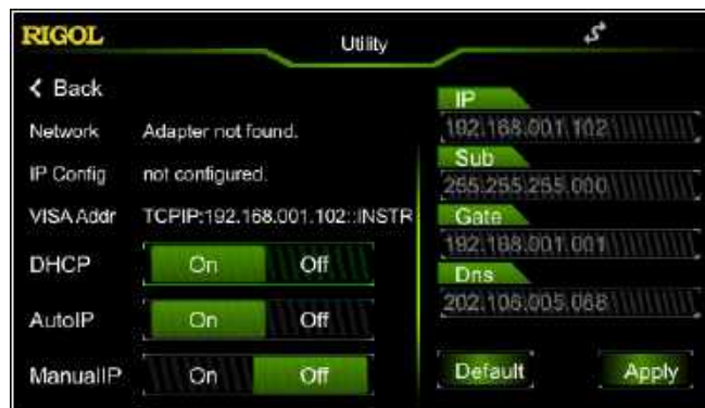
Figure 2-26 LAN Setting Interface
