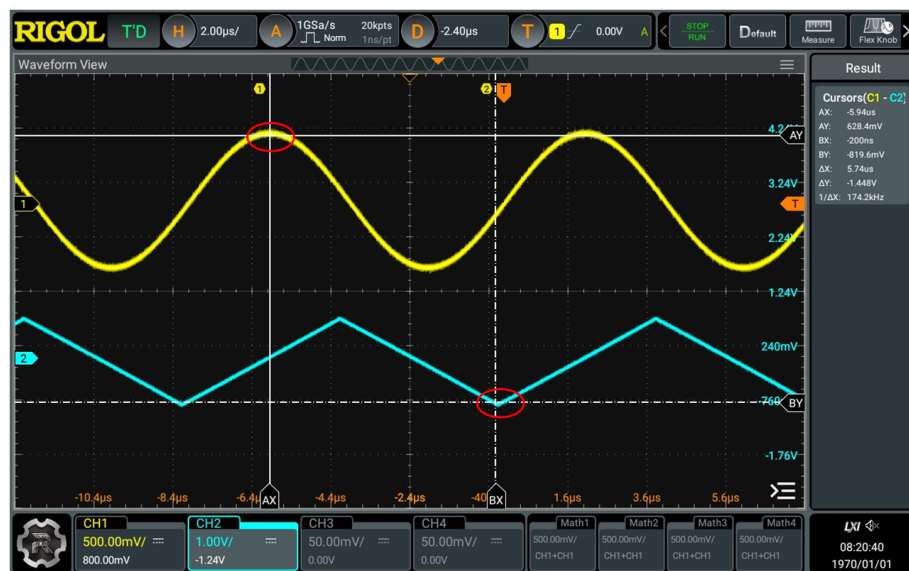
Figure 10.13 Track Measurement (after Horizontal Expansion)
