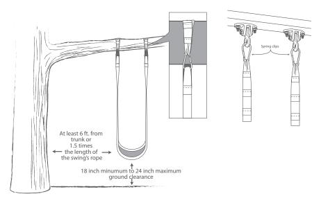
**LOOP** (TREE LIMB OR HORIZONTAL BEAM): Loop spring clips around limb (healthy, minimum 8 in. diameter) or beam and attach spring clip to a designated hanging loop on the same strap so swing seat when rider occupied is 18-24 in. above the ground surface.
