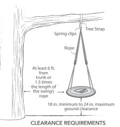
TREE LIMB ASSEMBLY: Test tree limb to ensure that it will hold the weight limit of 350 lbs. safely. SWING SET OR OTHER HORIZONTAL BEAM ASSEMBLY: Attach swing to a swing set by removing two sets of swings from the existing swing set and attach the spring clips to the chain support hooks.
