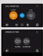
Through the **menu** you can constantly monitor the state of health of the machine, regulate and adjust, calibrate the balance (resetting to zero) use the Purge cycle
