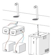
NOTE: When used with two control boxes, the POUR'D font can only dilute ONE syrup with water. The other syrup cannot be diluted with water.
