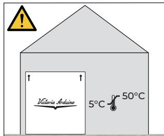
The package containing the machine must be stored away from atmospheric agents.
