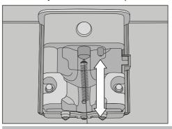
Push the cleaning brush a maximum of 1 cm into the steam jet.
