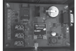
GSM MONITORS AND CONTROLS JVA ENERGIZERS USING A CELL PHONE
