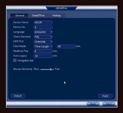
Clicking next will allow you to setup the basic network features of the recorder. We would recommend setting the network mode to "DHCP" to ensure your recorder connects automatically to your local network. (You will need to have a network cable connected from your recorder to your router at this stage)
