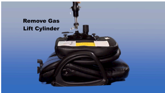
Illustration #10 Remove Gas Lift From Seat Plate.
