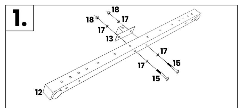
Placing one of the base frames on the side, secure the upright insert as shown in the picture above
