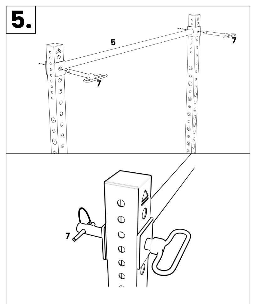
Insert the pin through the upright securing the pull up bar in place slide the pin lock into the back on the pin once in desired location
