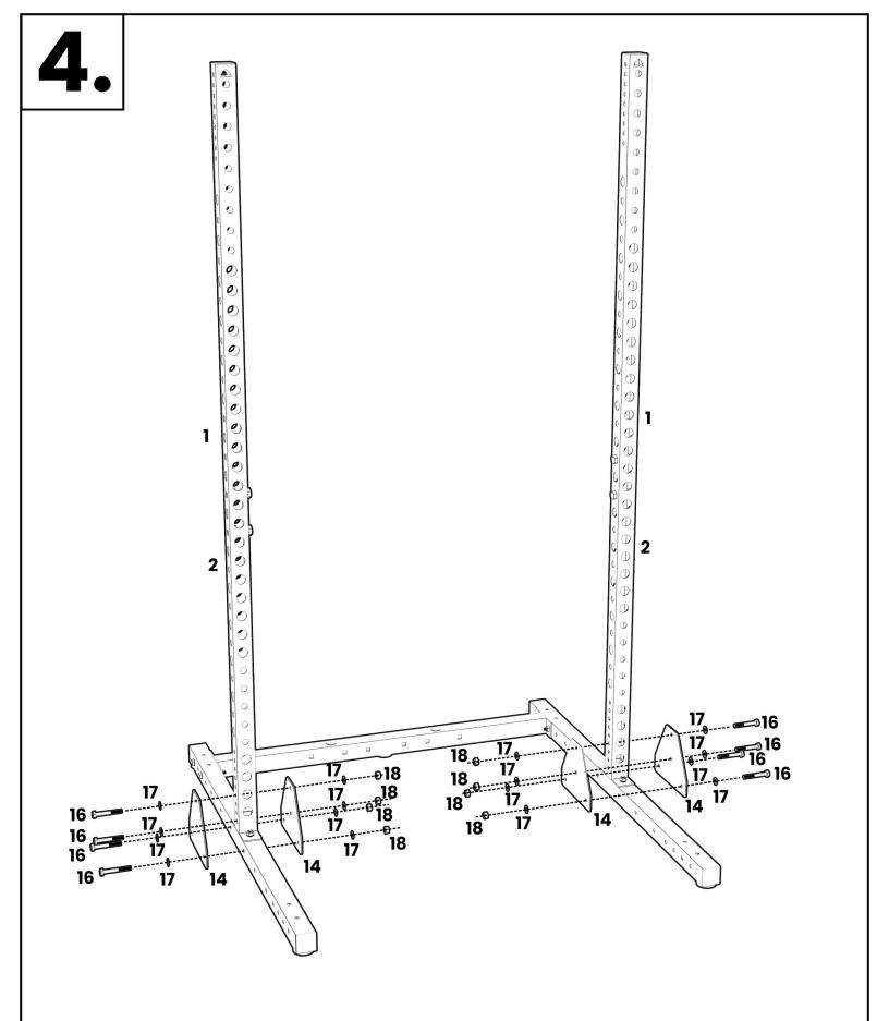
Align the triangle frames to the lower stabilizers and over the upright insert as pictured above. and secure using the included nuts, bolts, and washers.
