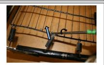
TWIST THE SCREWDRIVER SO THAT THE BLADE FORCES THE HOOK CLEAR OF THE WIRE AND THEN LEVER IT CLEAR OF THE WIRE FRAME. CARE!! – THE SPRINGS ARE UNDER TENSION.
