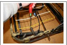
LEVER THE SCREWDRIVER FORWARDS (TAKE CARE NOT TO ALLOW THE SPRING OR SCREWDRIVER TO DISENGAGE FROM THE WIRE FRAME, AS IT WILL BE UNDER CONSIDERABLE TENSION)
