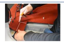
Now the carpet is fixed into place with the bolts, we can start to trim the steps – square off the back edge of the carpet using a knife.
