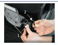
The handbrake switch is now accessible. With your thumb lift the catch and pull to remove the wire.
