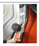
Once the flap has been turned the rubber excluder can be refitted - using a rubber mallet can make this a lot easier.
