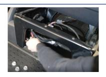
Next undo the 4, 17mm bolts from the base of the seat.
