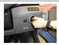
Now you will need to remove the light switch, turn the switch so it is on the '0'.
