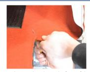
Now working on the edge at the front of the van – cut along the carpet from back to the front, this will allow the carpet to fold down easier.
