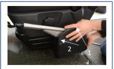
Lift the second remaining section up from the back and out over the handle. (This may require a slight wiggle or two)
