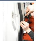
Once the B POST is clipped back onto the van you can pull out any rubber extrusion that maybe sitting underneath.
