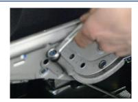
Undo the 10mm nut for the handbrake cable and remove
