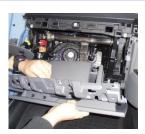
With the glovebox released disconnected any wires and remove from the van.
