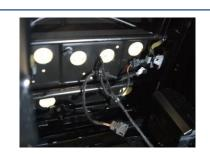
Unplug and remove any remaining wires that maybe attached to the bottom of the seat – the seat can now be removed from the van.
