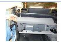
We can now start to remove the gloveboxopen the glovebox and then using a flat head screwdriver prize the top panel off.
