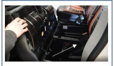
Pull forwards and remove the plastic cover then remove the electric connections. with a T20 Torx – place the box on the floor.
