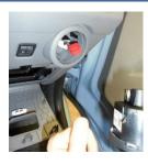
Pull the cable from the back of the switch and remove the screw in the base of the housing.
