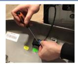
Now Repeat the last three steps on the passenger's side – if you have an electric switch this will need to be removed with a flat head screwdriver.
