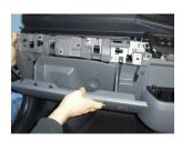
Open the glovebox again and pull forward to release the top from its clips.
