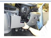
The driver's side lower dash can now be unclipped and pulled forward, remove any attached wires, and remove from the van.
