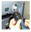
Push the centre of the switch in and turn one click to the right, this should now release the whole unit so it can be pulled free from the dash.
