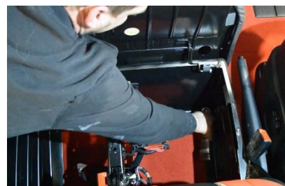
Refit the 8, 17mm bolts to the base of the bench seat – or the 4, 17mm bolts if you have a normal seat.
