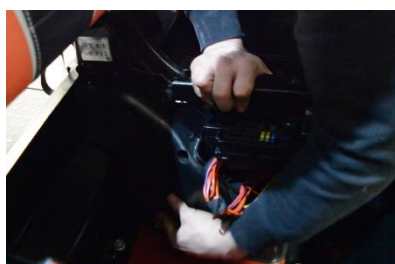
Reattached the plastic surround over the second wire loom.
