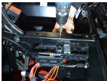
Reattached the wire loom to the frame with the T20 Torx.
