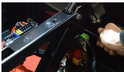
Reattached the second wire loom to the frame with the T20 Torx.
