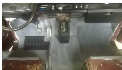
After the clips are fitted the main carpet area is complete.
