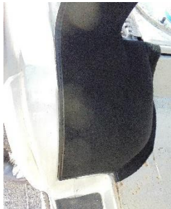
Fit the carpet from the front to back. Gently keeping the bound edge next to the groove in the wheel arch.
