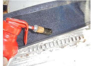
Then glue the back of the wheel arch carpet along the banded edge.
