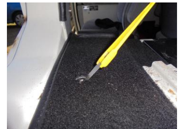
Locate the seat anchorage point hole and carefully cut the hole to allow for the bolt to go back through.
