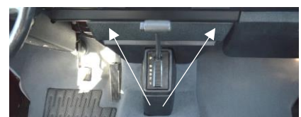
Fit the carpet set over the steering column and make a small incision in the carpet for the carpet fixing stud to come through. Then fit the plastic cover on top.
