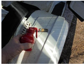
Firstly, glue the inside edge of the wheel arch. This creates a good bond for the carpet.
