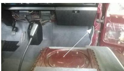
Pinpoint any fixing that would have been removed from the original carpet and then make the incisions ready for the clips to be reused and refitted.
