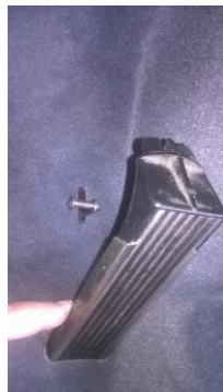
Feed the accelerator pedal through the carpet and reattach to the throttle pin.
