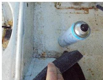
Once you are happy with the fit, you can then use the spray glue to fit the rest of the wheel arch carpet.
