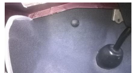
Fit the carpet set over the steering column and make a small incision in the carpet for the carpet fixing stud to come through. Then fit the plastic cover on top.
