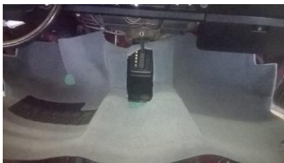
First you will need to feed the main carpet set over the gear lever.
